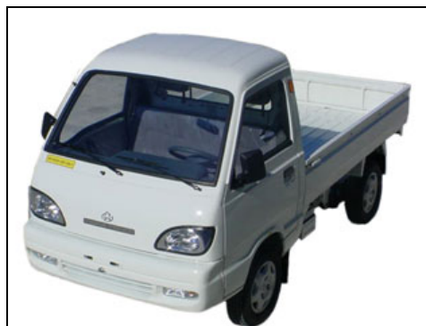
The mini Freight Village concept involves a cooperative effort between freight shippers and the City to centralize deliveries and transfer smaller goods to smaller vehicles to quickly and efficiently move goods to buildings. At just 55-inches wide and 11 ft. long, this example electric vehicle can carry 1,200 lbs. over 24 miles using alleyways, and on-street loading zones to make faster deliveries without taking up space and blocking streets.
