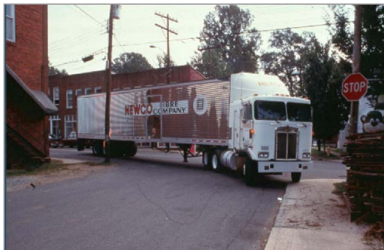
Primary and secondary freight streets require wider lanes and larger turning radii at intersections to accommodate heavy vehicles.
