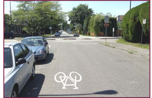
An example of a bicycle boulevard. Bicyclists are allowed to pass through this intersection, but vehicles must turn right.
