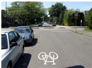
When it is not feasible to include exclusive bike lanes, desirable bicycle routes will be signed with bicycle route markers and marked with pavement markings.
