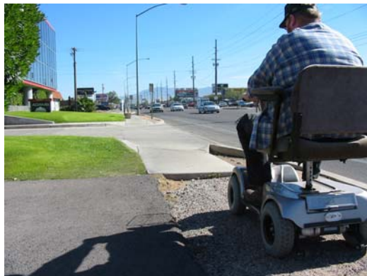
Figure 3. Although usable by most pedestrians, hard-packed dirt surfaces are not considered accessible sidewalks.
