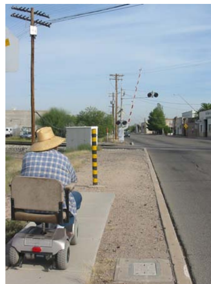
Figure 1. A gap in the sidewalk network makes this roadway inaccessible to wheelchair users.
