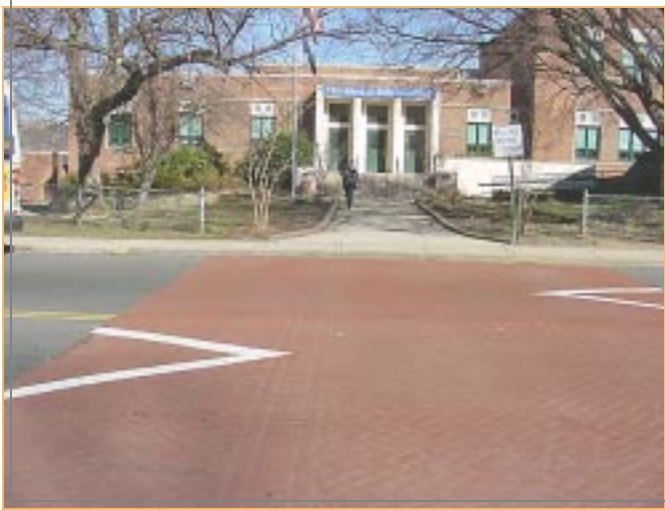
Speed table with stamped asphalt.
